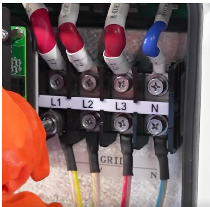
Figure 7-28 Grid port position of inverter
