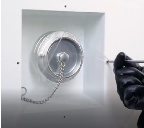
Figure 7-46 Remove the water inlet cover
