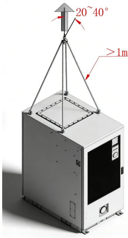
Figure 5- 7 Lifting Installation requirement
