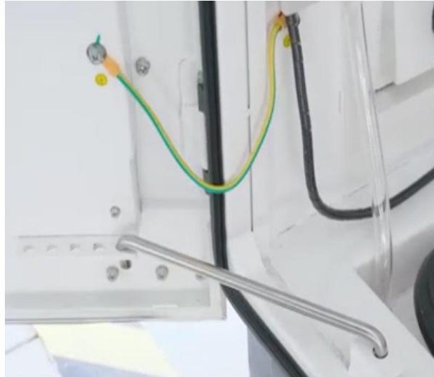
Figure 7-10 Cabinet Door stopper position
